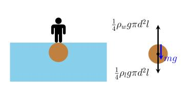
Solution: The volume of the log is  $V = \pi d^2 l/4$  and hence its weight is  $m_l g = \rho_l V g = \rho_l g \pi d^2 l/4$ . This weight, together with the weight mg of the person, are the two downward forces acting on the log. They are balanced by the upward buoyancy force,  $F_b = \rho_w V g = \rho_w g \pi d^2 l/4$ , where  $\rho_w$  is the density of water. Hence we can write
