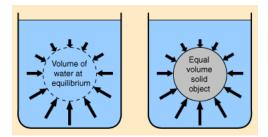
Fortunately there exists a simple and ingenious argument, which is attributed to Archimedes. The diagram shows an object submerged in the liquid (right) and an imaginary volume of liquid of exactly the same shape in place of the object (left). We now note that the forces pushing from the liquid at different depths are the same whether an object or a volume of the liquid is present. Hence the volume of the liquid experiences exactly the same buoyancy force as the object.
