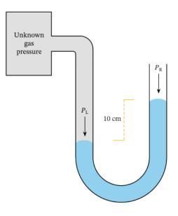
A liquid column manometer contains fresh water,  $\rho_w = 1000 \text{ kg/m}^3$ . The left side is connected to a gas of unknown pressure, and the right side is open to the atmosphere at sea level, with pressure of 101.3 kPa. Determine the absolute pressure of the unknown gas.
