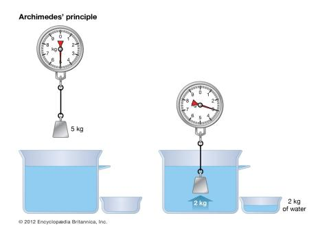
The above image demonstrates that putting the mass into liquid reduces the reading on the scale by 2kg. This means the buoyancy force is approximately equal to  $2 \text{ kg} \times 9.81 \text{ N/kg} = 19.6 \text{ Newtons}$ . This also means that the weight of the displaced liquid is equal to 19.6 Newtons.
