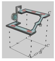
This means that the equivalent resistance of the two resistors in series is simply the sum of their resistances:  $R_T = R_1 + R_2$ .
