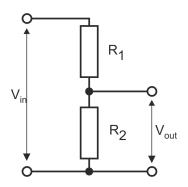
Solution. We have two resistors in series. As we know from Example 4, the current through the circuit is  $I = V_{\rm in}/(R_1 + R_2)$  and hence the potential difference on  $R_2$  is  $V_{\rm out} = IR_2 = \frac{R_2}{R_1 + R_2}V_{\rm in}$ .
