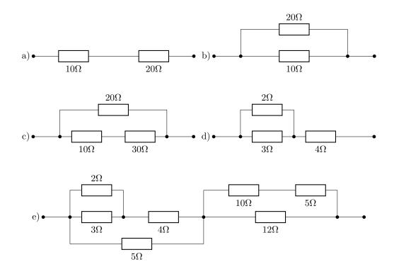
**Problem 4** (2 marks). An ideal voltmeter must have infinite resistance and should be connected parallel to the circuit element whose potential difference needs to be measurement. In contrast, an ammeter needs to be connected in series with the circuit element and should ideally have zero resistance. Explain why it is the case, using  $R_T = R_1 + R_2$  and  $\frac{1}{R_T} = \frac{1}{R_1} + \frac{1}{R_2}$ .
