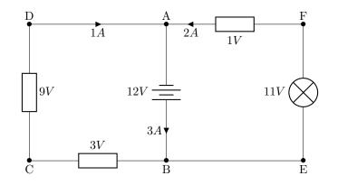
Solution. There are 3 loops in this circuit, for which KVL can be written: ABCD, ABEF and DFEC.
