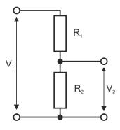
This problem demonstrates a shortcoming of the voltage divider as a variable voltage source. To avoid disrupting the output voltage, the load resistance must be much less than the two resistors making up the divider. But that means that most of the power will be wasted on these two resistances rather than the load. Therefore in practice other solutions are used to construct variable voltage sources — for example, variable transformers.
