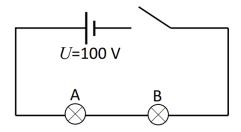
Consider the above circuit. The filament lamp A consumes an electrical power  $P_A = 100$  W when it alone is connected to a voltage of U = 100 V. Filament lamp B consumes a power  $P_B = 20$  W when it alone is connected to a voltage of U = 100 V.
