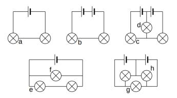
Determine whether the bulbs marked by letters in these circuits are brighter than normal, normal, dimmer than normal, or off.
