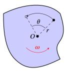
These parallels allow us to apply intuition and problem-solving techniques from linear motion to rotational motion. Assuming constant angular acceleration, the kinematic equations of rotational motion are very similar to the linear kinematic equations (SUVAT equations):
