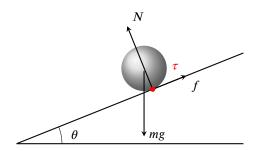
**Method 2**. Let us instead choose the sphere's centre as the axis. Now the torques of gravity and normal reaction forces vanish, but the friction has non-zero torque  $\tau = f R$ . This torque causes the acceleration
